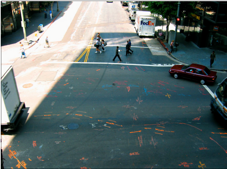
Figure 4.1: A road junction outside the One Wiltshire building, an internet hub in downtown Los Angeles, that is heavily marked with ‘utility graffiti’ signifying the location of underground cable routes leading into the building. Such markings are a kind of 1-to-1 map of the complexity of what lies unseen just beneath the surface. (Source: Varnelis 2002.)
