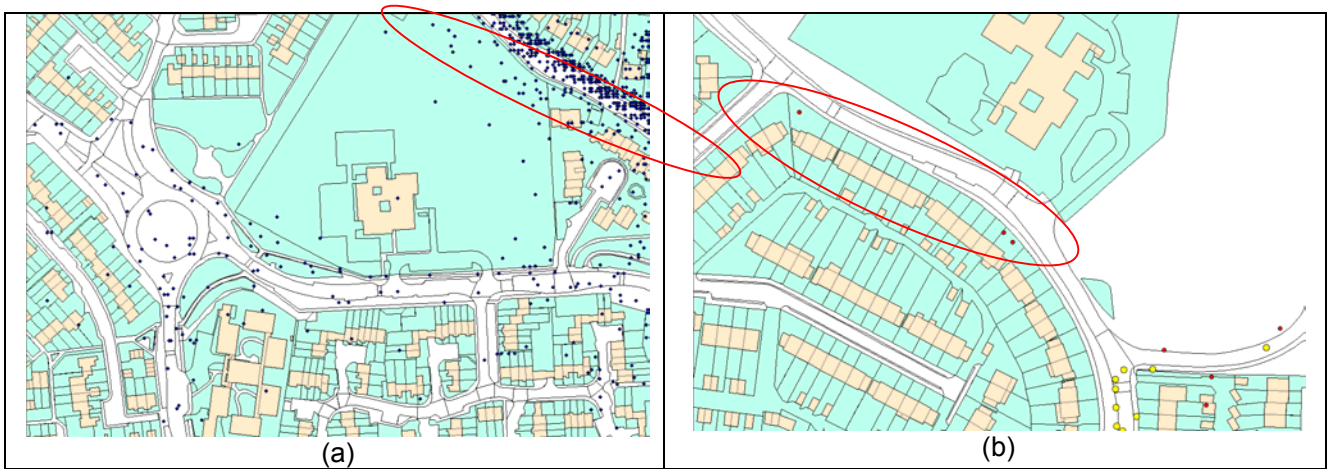
Figure 26 sample of GPS positioning errors (the dots within red circle are supposed to fall onto roads)
