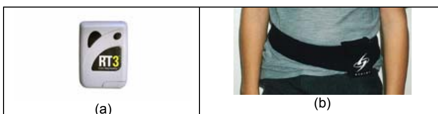
Figure 5 RT3 monitor (a) and a child wearing the monitor around his waist (b)
