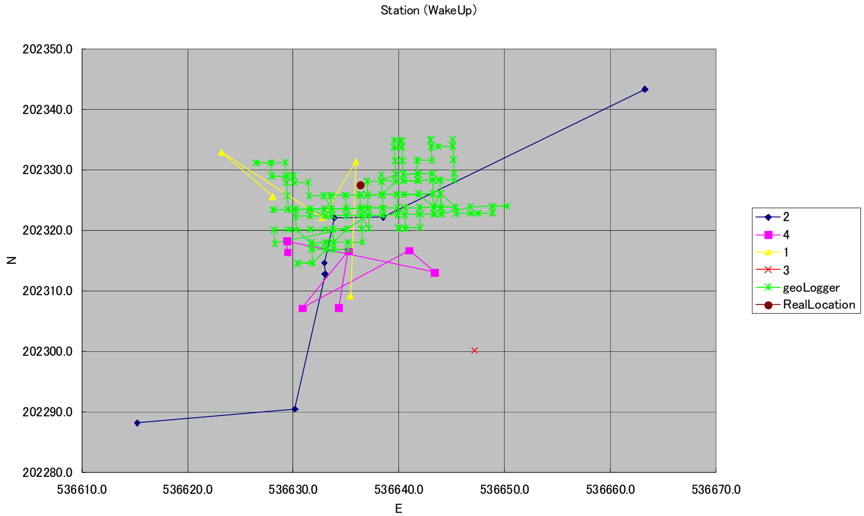
Figure 28 GPS Accuracy test :GPS location information from 5 GPS units under stationary condition.
