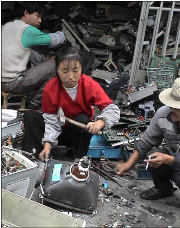
Dismantler cracking a monitor to remove the copper yoke. The rest of the CRT is dumped. © BAN
