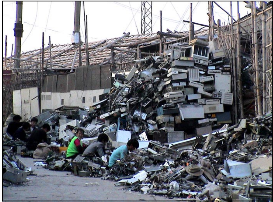
Very typical on-street E-waste dismantling operation in Guiyu. Using hammers and chisels and their bare hands, workers separate the waste into aluminum, steel, copper, plastic and circuit boards. © BAN
