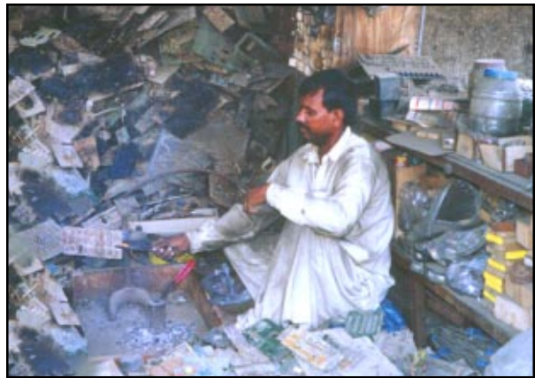
Worker de-soldering circuit boards with a Bunsen burner in Sher Shah. © SCOPE
