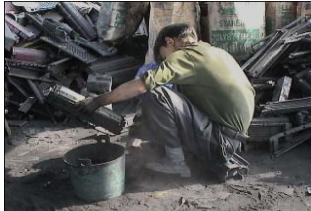
Worker without respiratory protection brushing carbon black toner from printer cartridge into bucket. © BAN
