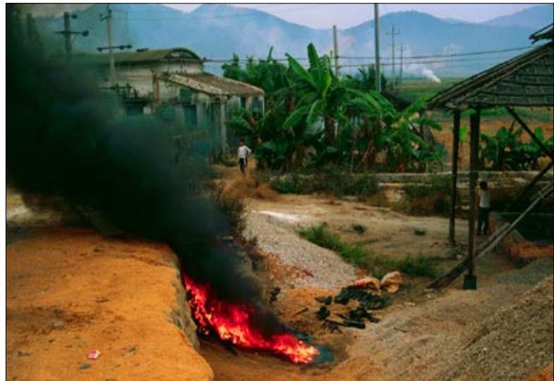
Open burning of wires and other parts are common to recover metals such as steel and copper. Dioxins and furans can be expected due to the use of PVC and brominated flame retardants. © BAN
