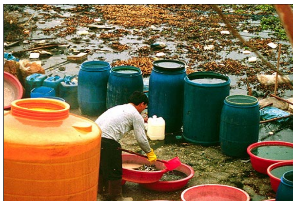
Laborer swirling aqua regia acid over computer chips to extract gold. © BAN
