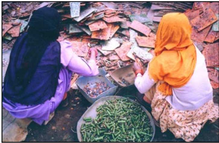
Women plucking components from circuit boards with pliers and wire cutters in New Delhi. © Toxics Link India
