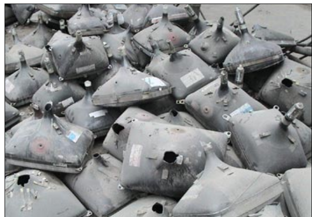
Broken CRTs awaiting land disposal after the copper yoke has been removed in Guiyu, China. © BAN
