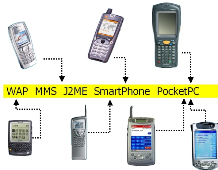
Figure 2.1 Examples of mobile devices and their protocols (WAP=wireless application protocol, MMS = Multimedia messaging, J2ME = Java2 Micro Edition), (based on Li and Maguire, 2003).
